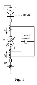
A restrained differential current protection is installed on a transformer (Fig.1). The operating characteristic is shown in Fig.2.
