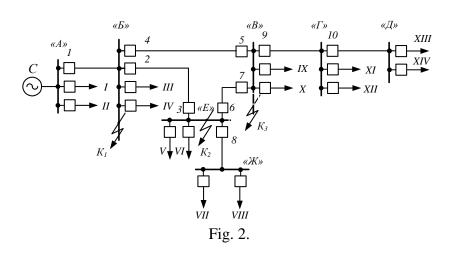
Source data:  $I^{(3)}_{KImax} = 2,8$  kA;  $I^{(2)}_{protection KImin} = 1,8$  kA;  $I_{overcurrentI}$ .  $I^{(2)}_{protection K2min} = 1,2$  kA;  $I^{(2)}_{protection K3min} = 0,63$  kA;  $I_{dynamic current}$  approach choice
