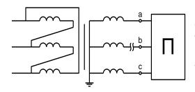
A symmetrical three-phase resistive receiver which phases are connected in a "triangle" is connected to the secondary winding of the transformer ( $\Delta$ /Y) 6,0/0,38 kV. P<sub>receiver</sub>=6 kW. Determine the values of a, b and c potentials relative to the
