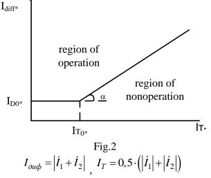
Minimum operating current  $I_{D0*} = 0,3$  pu
